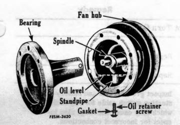
10. Turn the fan hub so the oil retainer screw is at a right, horizontal position. Remove the screw and fill the hub with lubricant. (Refer to Operator's Manual.)
