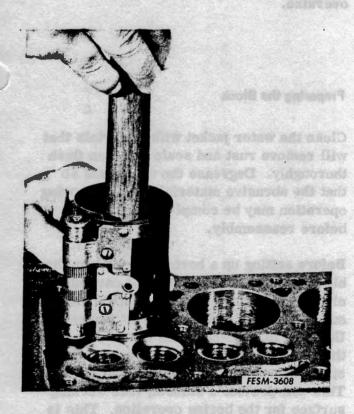
NOTE: When reinstalling a piston and connecting rod assembly, install the assembly in the same cylinder bore and in the same position from which it was removed. Connecting rods are stamped with the cylinder number on one side of the rod and on the same side of the bearing cap, No. 1 starting at the front end of the engine. Be sure to install the numbered side of both the rod and bearing cap so both are on the camshaft side of the engine.
