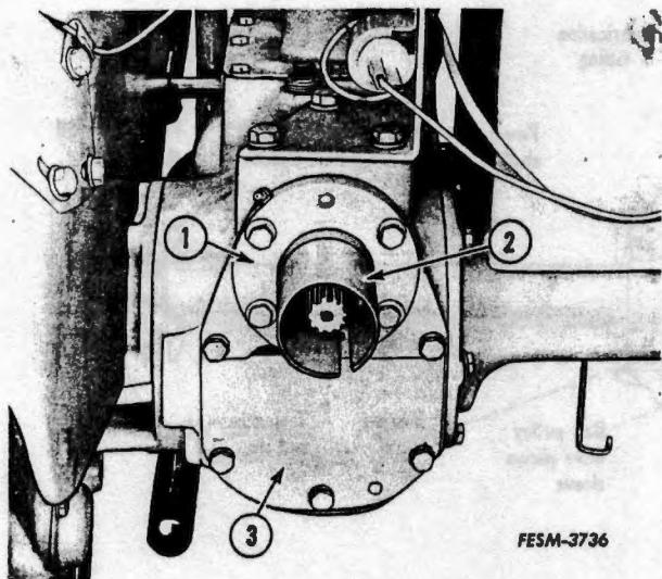
1. Remove the belt pulley assembly if equipped.
