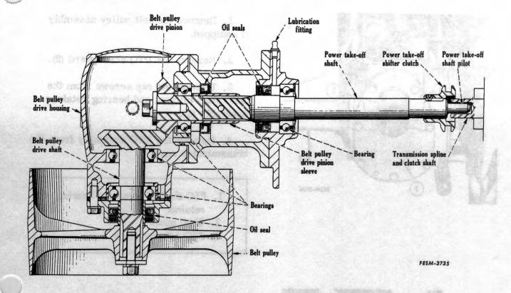
1. Install the drive shaft and inner bearing in the drive housing.
