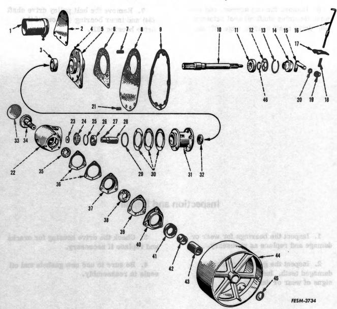
1. Remove the belt pulley assembly from the PTO assembly and drain the lubricant from the drive housing.
