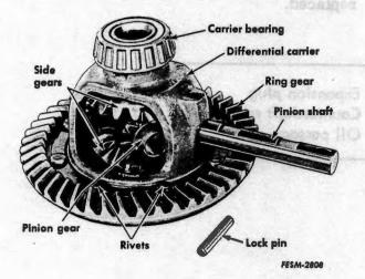
2. Assemble the side gears and the pinion gears in the differential carrier.
