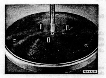
1. Place the three, round, one inch blocks on the plate of the clutch service tool, FES 50.
