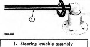
1. Inspect the axle pivot shaft, thrust washers and bushings for wear or damage. Replace as necessary.
