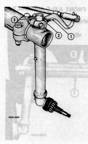
5. Remove the steering knuckle arm (1) from the steering knuckle (3), and remove the key (2) from the steering knuckle.
