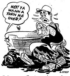
If the tractor will not move because the rear wheels have dug in or sunk deeply into the ground, don't fasten logs, posts, or anything to the rear wheels that will prevent them from rotating. This would be certain to tip the tractor over backward. Instead......
