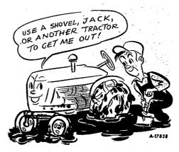
......dig out or jack up the rear wheels and fill in under them. Or, if another tractor is available, hitch it with a chain to the front end of the "stuck" tractor. The power of both tractors can be used, if needed, provided a heavy pull is kept on the chain all the time.
