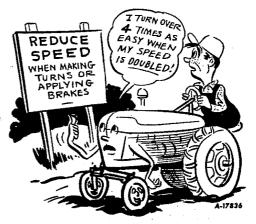
Reduce speed before making a turn or when applying the brakes. Remember, the danger of the tractor overturning increases four times when the speed is doubled.
