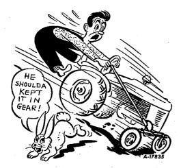
Always keep the tractor in gear when going down steep hills.
